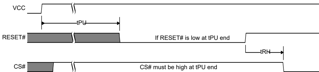
Figure 136. Reset low at the end of POR
