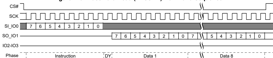
Figure 115. Password Read (PASSRD) Command Sequence
