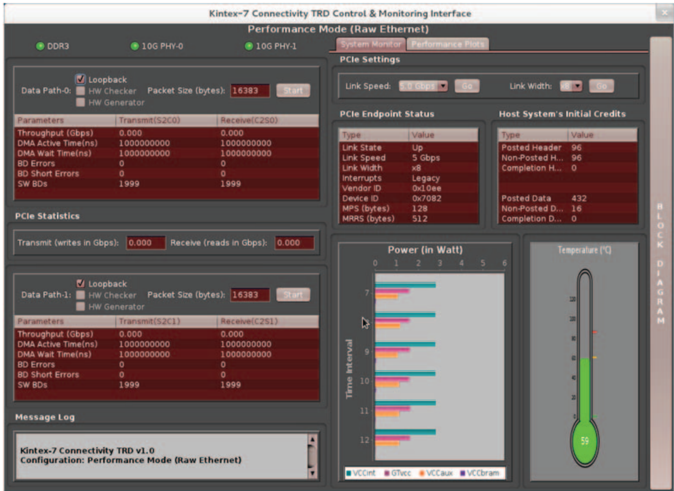
Figure 2-23: Raw Ethernet Driver GUI
