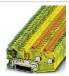
Feed-through terminal block, Connection type: Quick connection, Spring-cage connection, Cross section: 0.5 mm² - 2.5 mm², AWG :20- 14, Width: 6.2 mm, Color: green-yellow, Mounting: NS 35/7,5, NS 35/15
