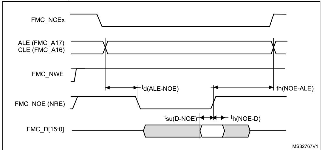
Figure 34. NAND controller waveforms for write access
