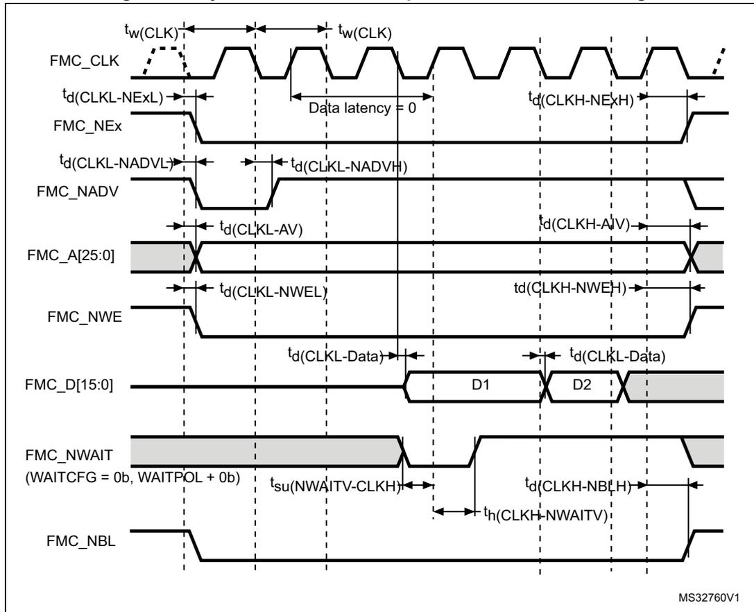
**Table 68. Synchronous non-multiplexed PSRAM write timings<sup>(1)</sup>**
