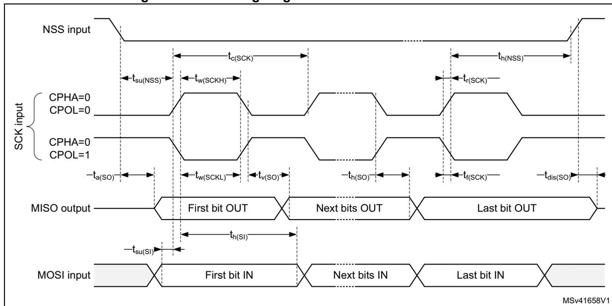
Figure 47. SPI timing diagram - slave mode and CPHA = 1<sup>(1)</sup>
