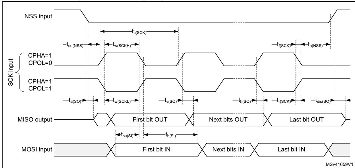
1. Measurement points are done at  $0.5 \times V_{DD}$  and with external  $C_L = 30$  pF.
