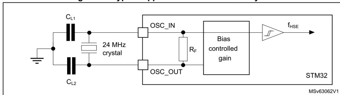
**Low-speed external clock generated from a crystal/ceramic resonator**
