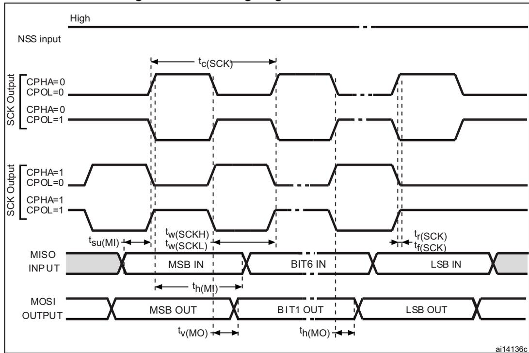
1. Measurement points are done at  $0.5 \times V_{DD}$  and with external  $C_L = 30$  pF.
