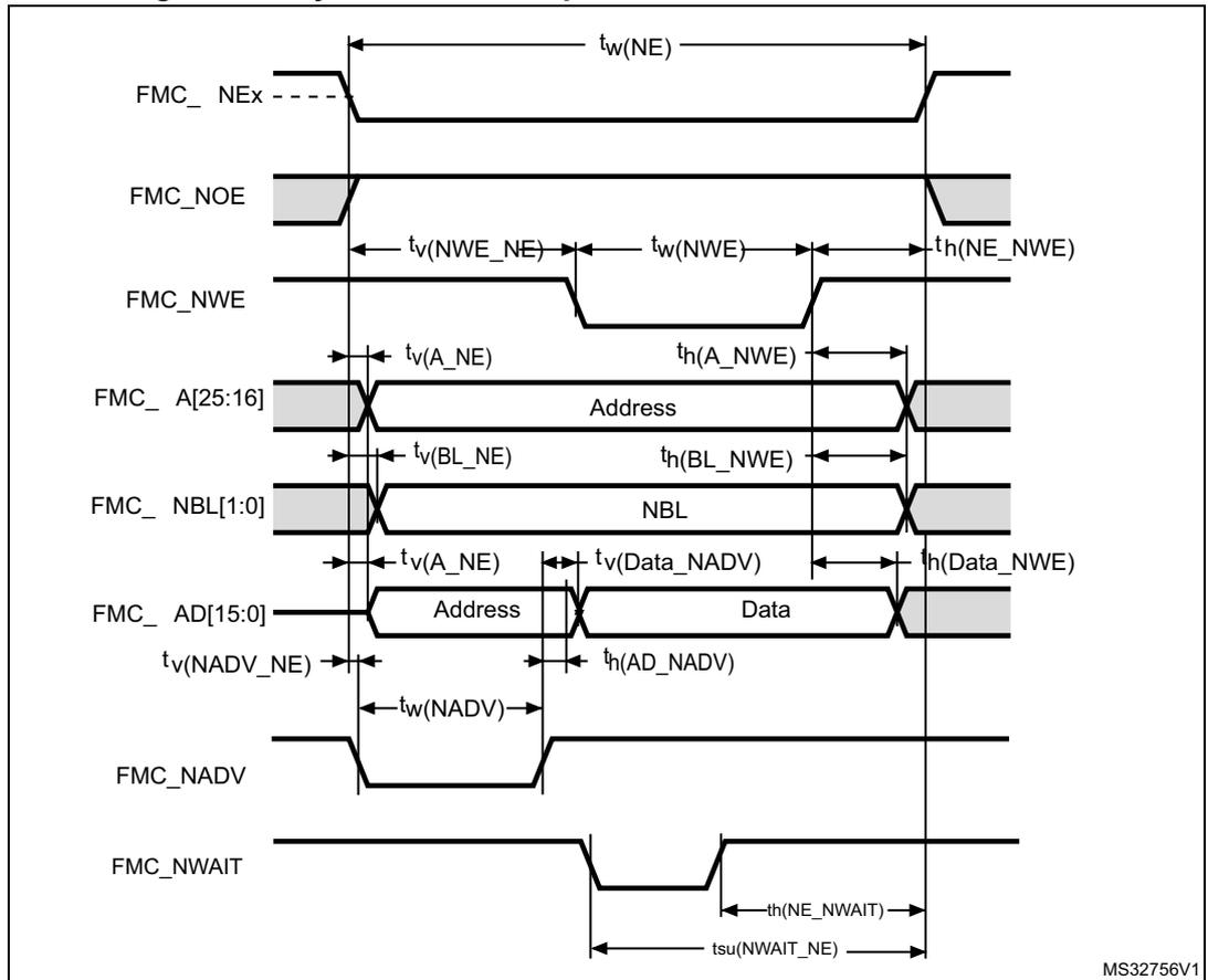
**Table 63. Asynchronous multiplexed PSRAM/NOR write timings<sup>(1)</sup>**
