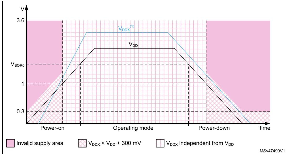
1.  $V_{DDX}$  refers to any power supply among  $V_{DDCORE}$ ,  $V_{DDA}$ ,  $V_{DDA1V8\_REG}$ ,  $V_{DDA1V1\_REG}$ ,  $V_{DD3V3\_USBHS/FS}$ ,  $V_{DDQ\_DDR}$ .
