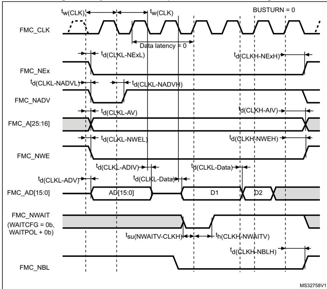
**Table 66. Synchronous multiplexed PSRAM write timings<sup>(1)</sup>**
