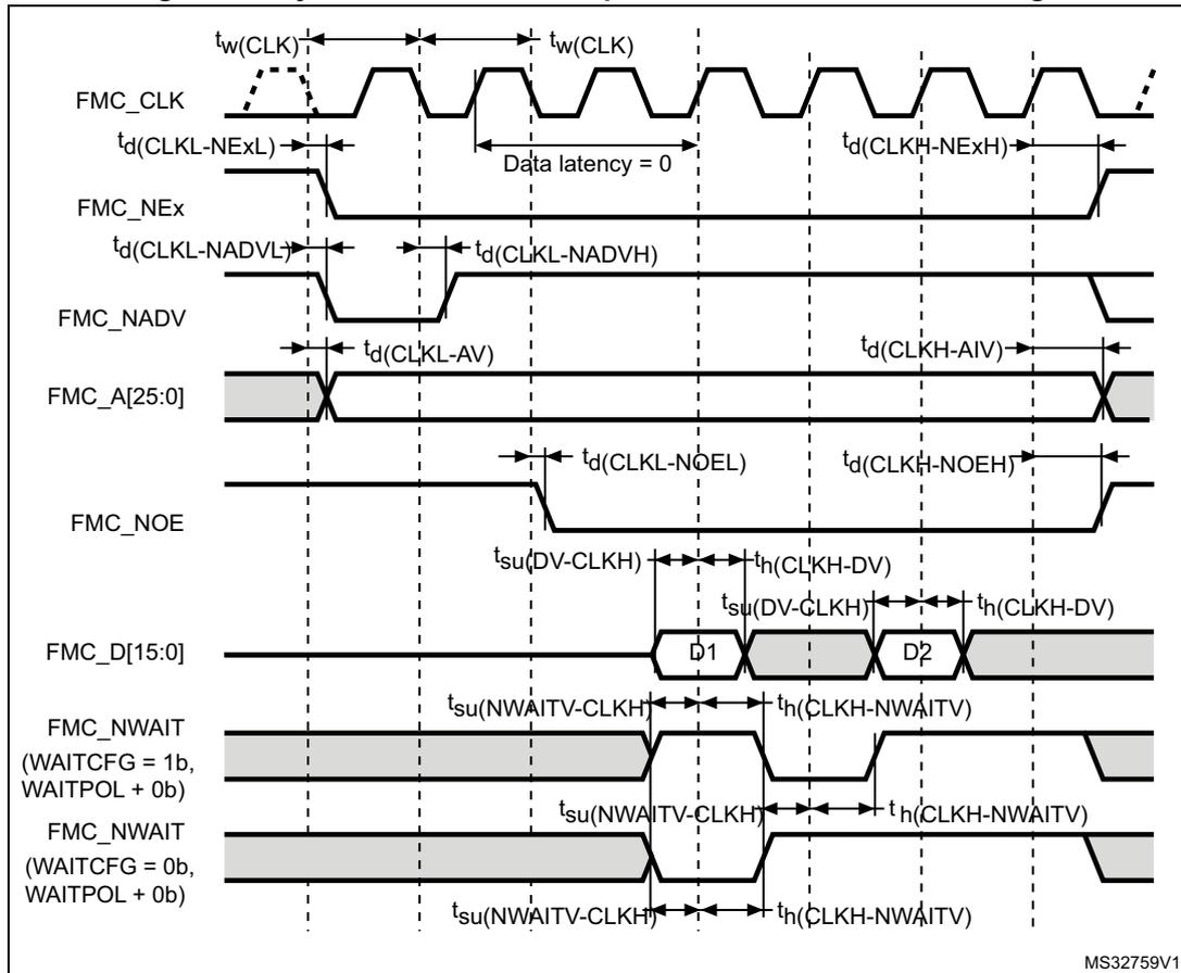
Table 67. Synchronous non-multiplexed NOR/PSRAM read timings<sup>(1)</sup>
