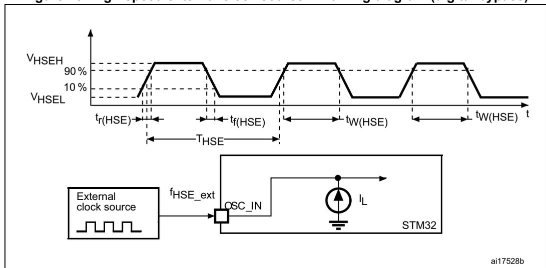
**Table 29. High-speed external user clock characteristics (analog bypass)<sup>(1)</sup>**
