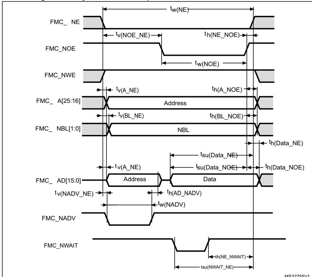
**Table 61. Asynchronous multiplexed PSRAM/NOR read timings<sup>(1)</sup>**
