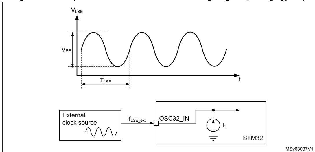
**Low-speed external user clock generated from an external source**
