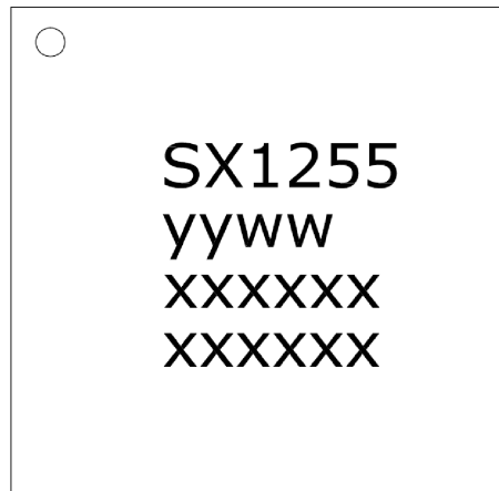
Figure 7-3: SX1255 Marking Diagram
