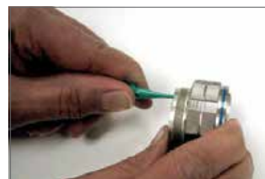
Plastic tool with contact in proper position.
