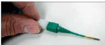
Plastic tool with contact in proper position.
