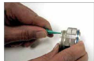
Plastic tool with contact in proper position.
