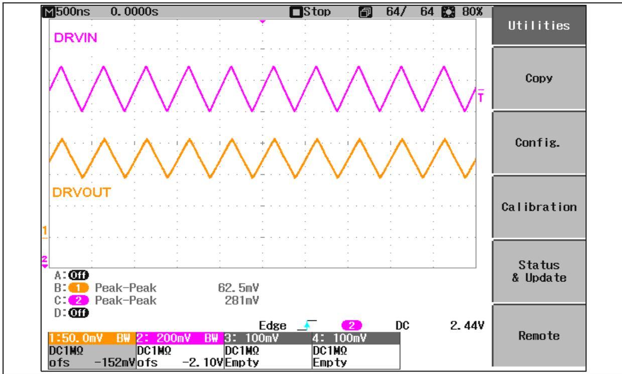
FIGURE 5-2: Inductor Driver Transfer Function ( $R_{load} = 100 \text{ Ohm}$ )
