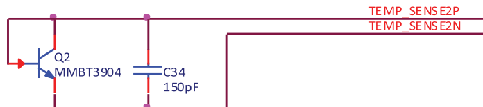
Figure 8.5. NPN Temperature Sensor Circuit
