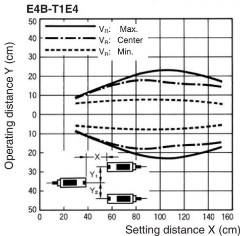
**Note:** Obtain the point that turns  $Y_1$  and  $Y_2$  ON while changing the sensing distance (X).
