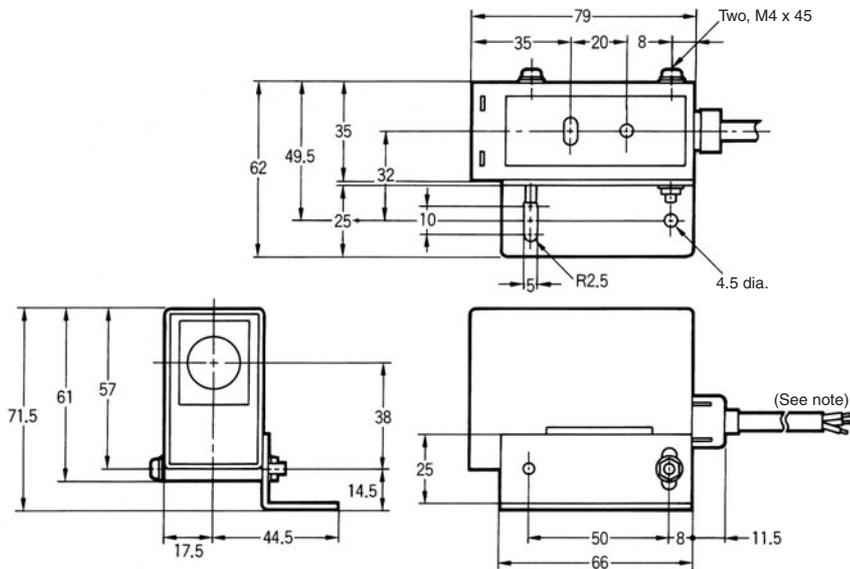
**Note:** Vinyl-insulated round cord with three conductors, 6 dia.; standard length: 2 m
