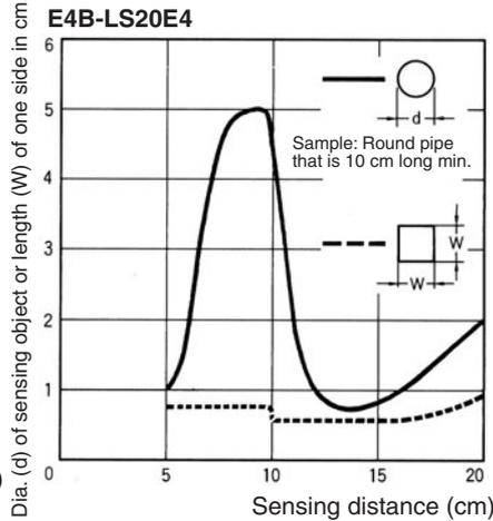
**Note:** The sensing method will change when the sensing distance exceeds 10 cm. As a result, the detectable diameters will change greatly.
