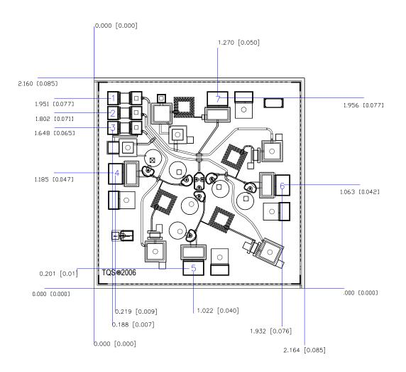
Units: millimeters (inches) Thickness: 0.100 (0.004)
