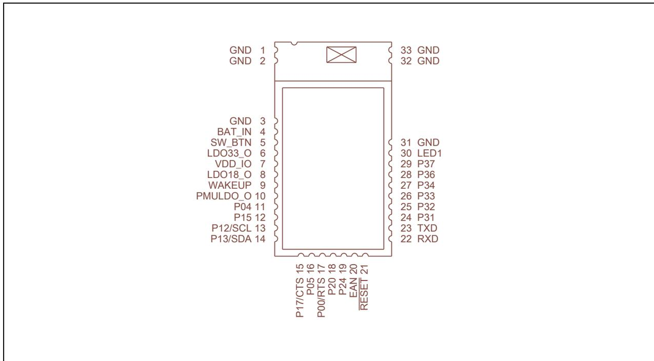
**FIGURE 1-3: BM77SPP03MC2 PIN DIAGRAM**
