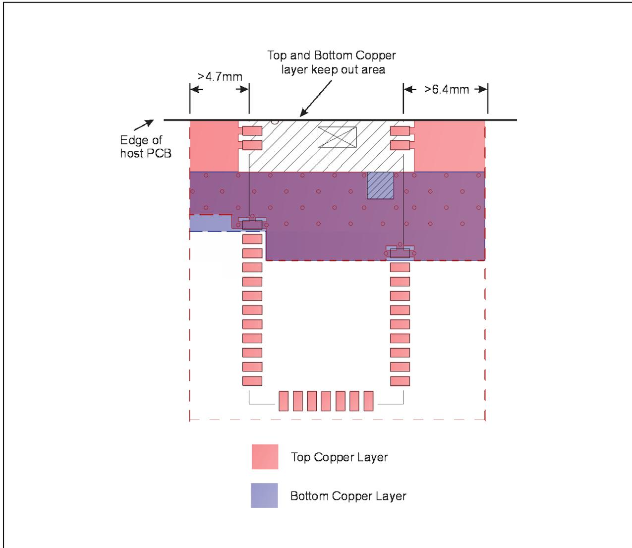
**FIGURE 1-9: BM77SPP03MCS MODULE DIMENSIONS**
