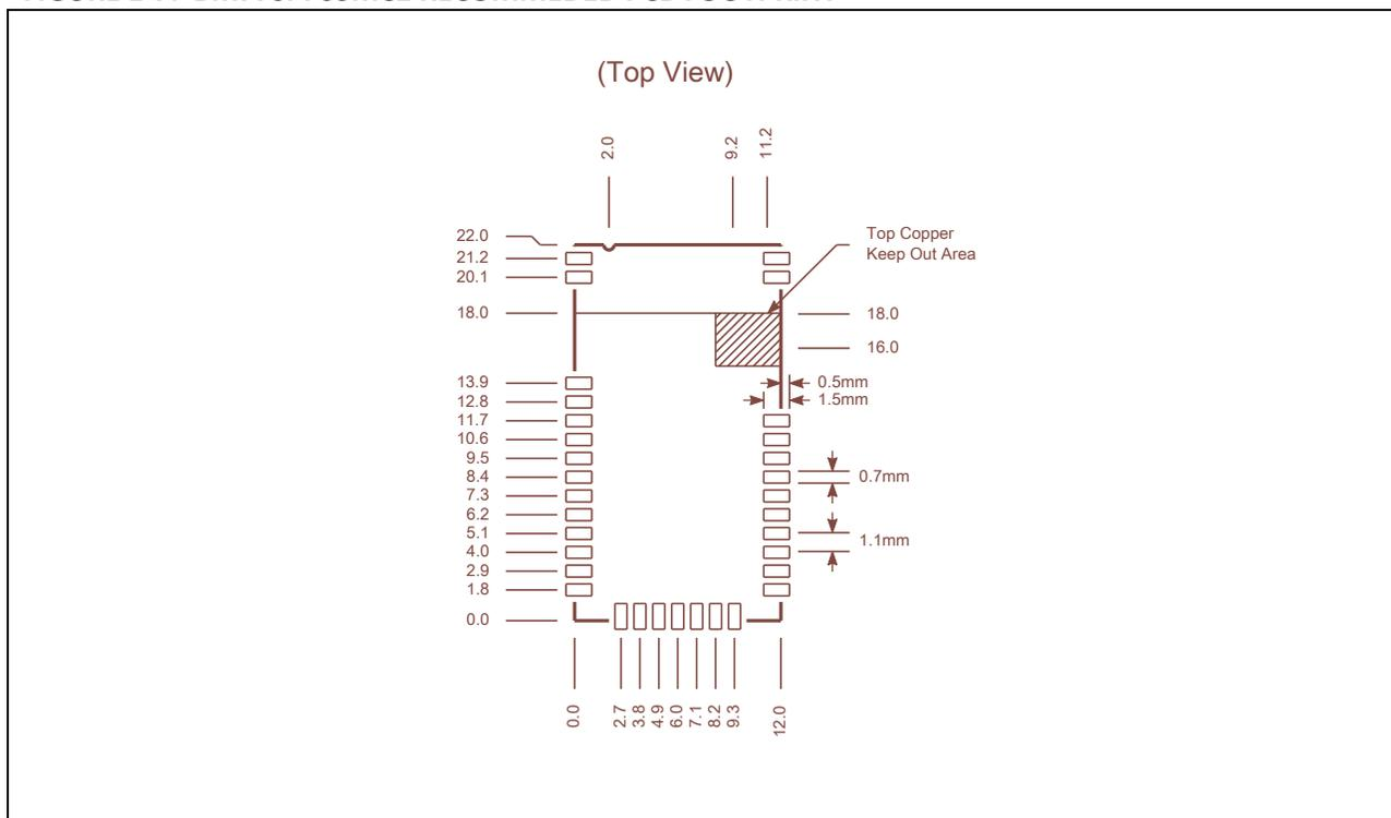
FIGURE 1-8: BM77SPPS3MCS HOST PCB MOUNTING SUGGESTION
