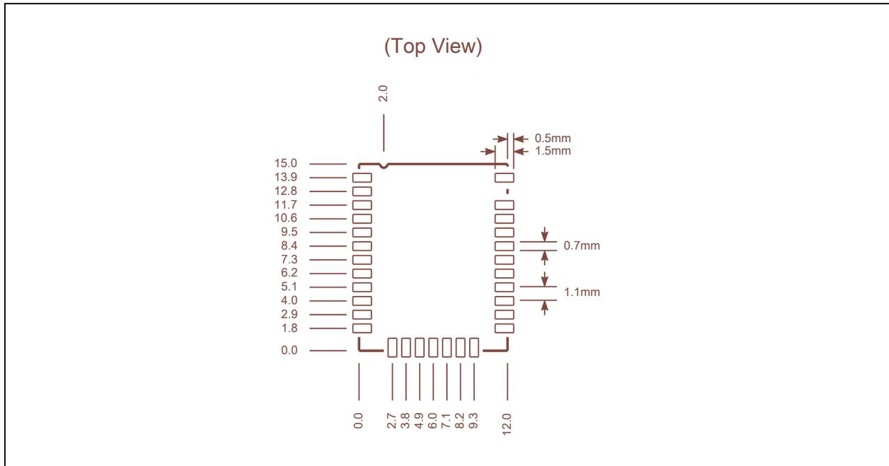
FIGURE 1-11: BM77SPP03MCS HOST PCB MOUNTING SUGGESTION
