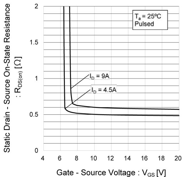
Fig.11 Static Drain - Source On - State
