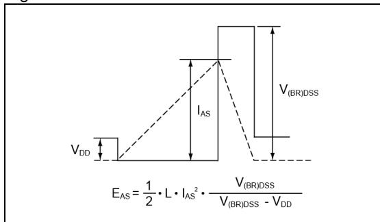
Fig.4-2 dv/dt Waveform
