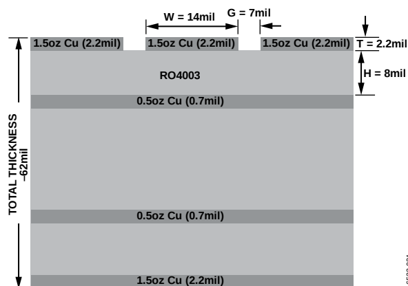
Figure 22. Probe Matrix Board (Cross Section View)
