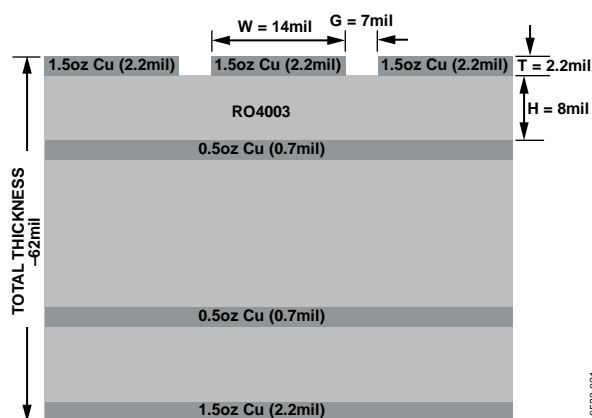
Figure 22. Probe Matrix Board (Cross Section View)
