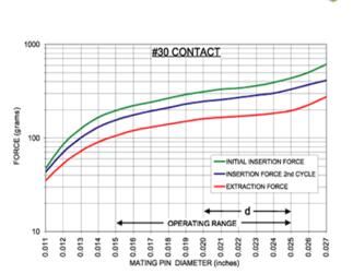
The insertion/extraction/normal force characteristics above were derived using a 30 microinch gold plated contact and polished steel gauge pins having a bullet-shaped tip.
