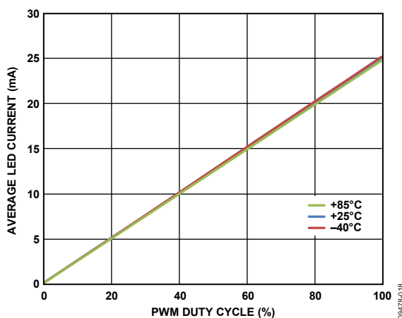
Figure 18. Typical Average I_{OUT} vs. PWM Duty ( f_{PWM} = 300 Hz)
