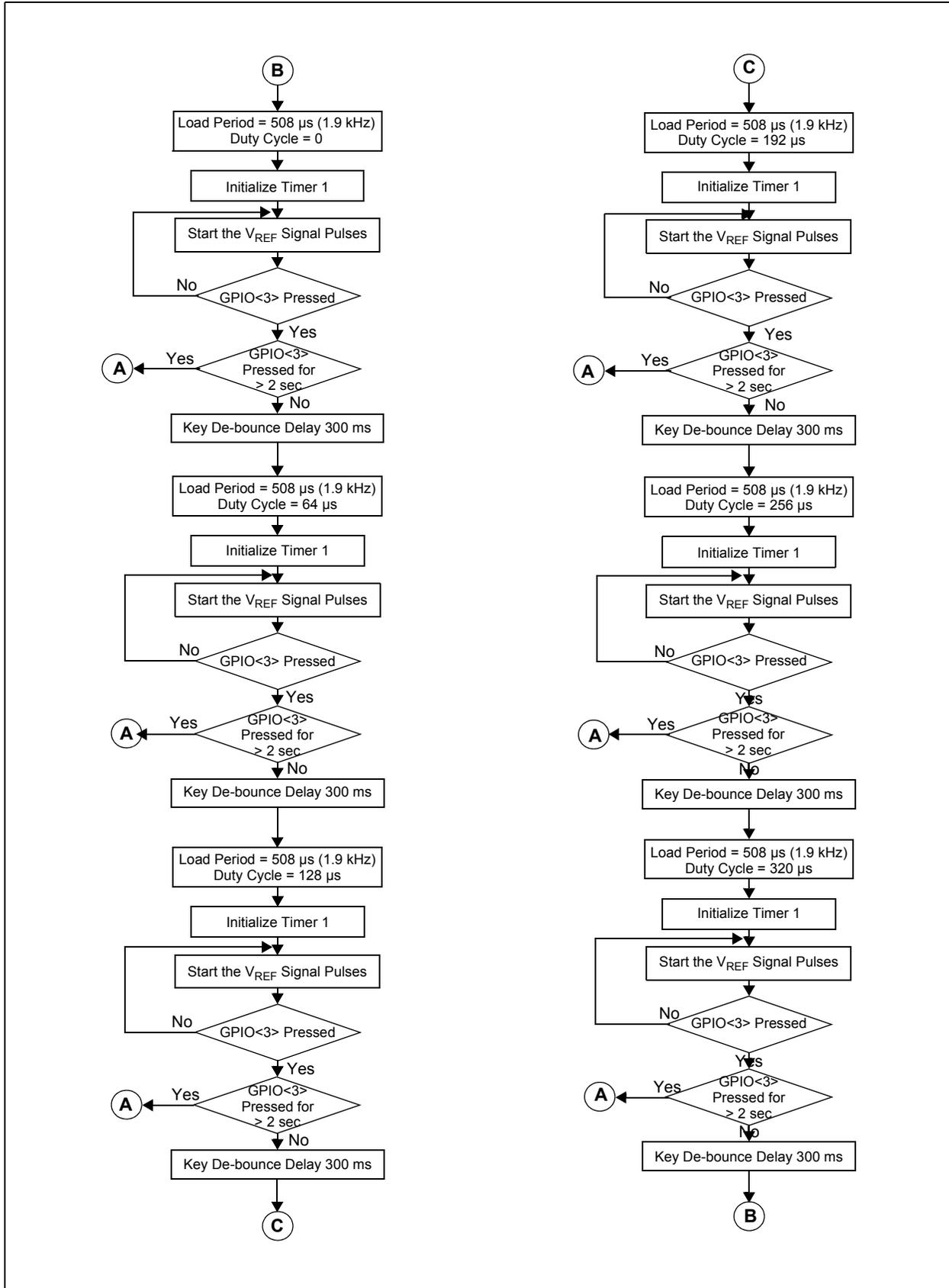
**FIGURE C-1:** Firmware Flowchart.
