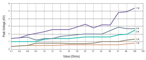
1.2/50  $\mu s$  Peak Voltage Limit (10 pulses at 10 sec. intervals,  $\Delta R < 5$  %)
