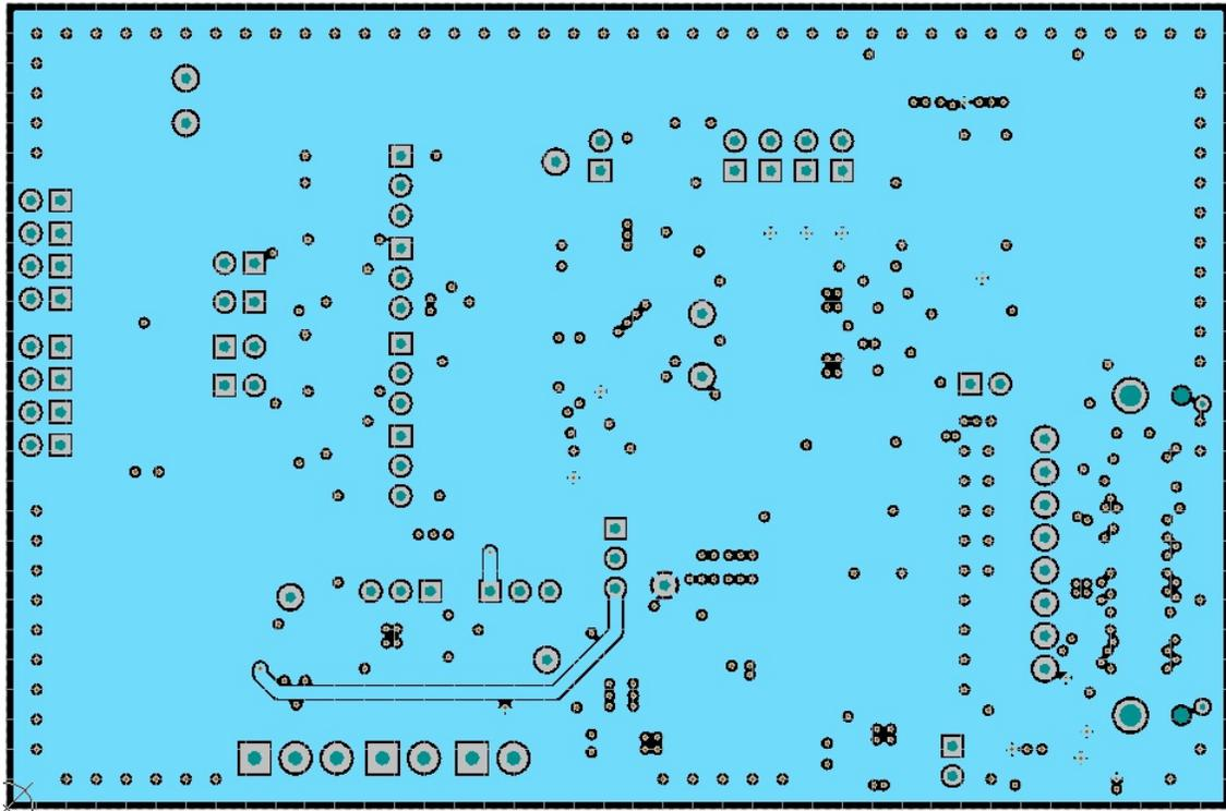
Figure 33. ADS86xxEVM PCB: Digital Power Layer (L4)
