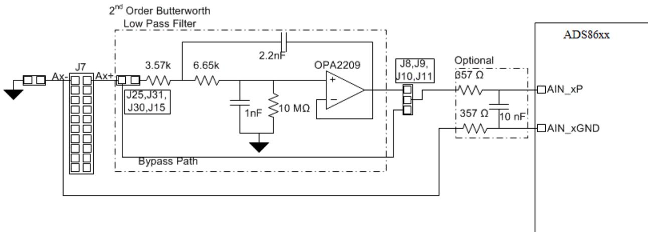
Figure 1. ADS86xxEVM Analog Input Connections for Channels AIN0, AIN1, AIN2, and AIN3
