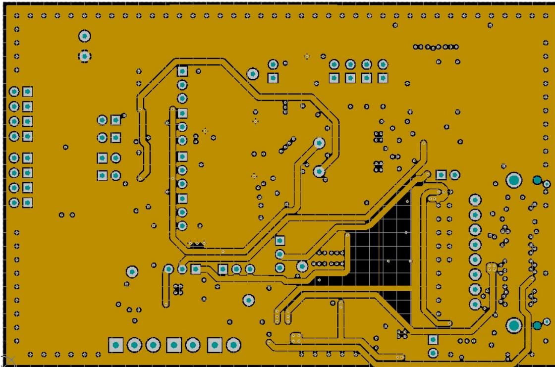
Figure 32. ADS86xxEVM PCB: Analog Power Layer (L3)
