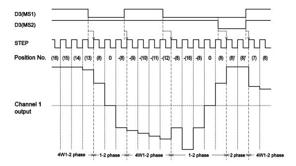
If the excitation mode is switched when power is applied to the motor, the operation follows the sequence shown below. (CW mode)
