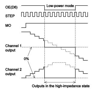
When the OE bit in the serial data, D6 (100, \*\*\*, D6, \*), is set to 0, the output is turned off and set to the high-impedance state at the rise of STB.
