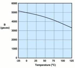
Measured on an 18/10/6 mm toroid at 10kHz and H=5 oersted.
