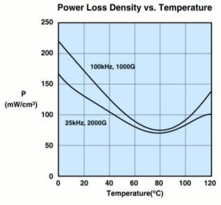
Measured on an 18/10/6mm toroid using the Clarke Hess 258 VAW.
