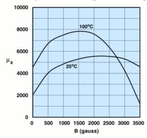
Measured on an 18/10/6mm toroid at 10kHz.
