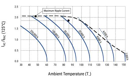
Axial Aluminum Electrolytic Capacitors - PEG126, +150°C
