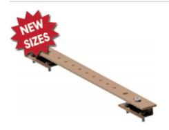
The GRDBAR Series comes in vertical, horizontal mounting as well as horizontal rack mounting. The grounding bar is made from heavy-gauge copper that attaches to the inside of an enclosure, cabinet or open frame rack to provide consolidated equipment grounds. Ground points have been drilled and tapped to accommodate a #10-32 screw (included). Use with our **Ground Wire Kits** to bond your equipment to the busbar.
