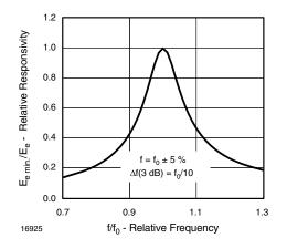
Fig. 5 - Frequency Dependence of Responsivity
