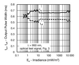
Fig. 4 - Output Pulse Diagram
