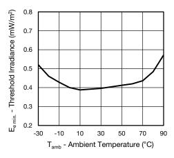
Fig. 6 - Sensitivity vs. Ambient Temperature
