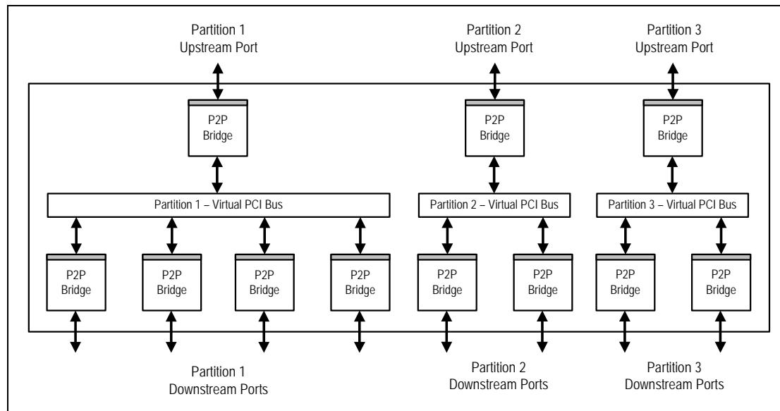
Figure 2 Example of Usage of Switch Partitioning
