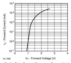
Fig. 3 - Pulse Forward Current vs. Forward Voltage
