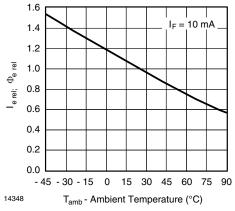
Fig. 7 - Relative Radiant Intensity vs. Ambient Temperature
