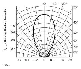
Fig. 9 - Relative Radiant Intensity vs. Angular Displacement
