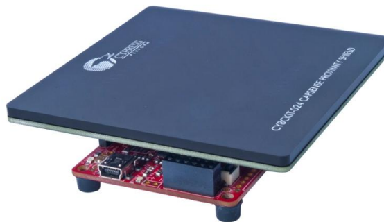
Figure 1-3: CY8CKIT-024 Connected to CY8CKIT-042
