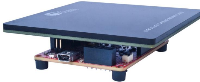
Figure 1-3: CY8CKIT-024 Connected to CY8CKIT-042
