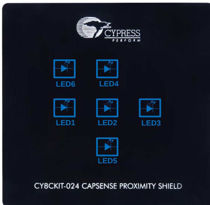
Figure 2-14: LEDs on CY8CKIT-024
