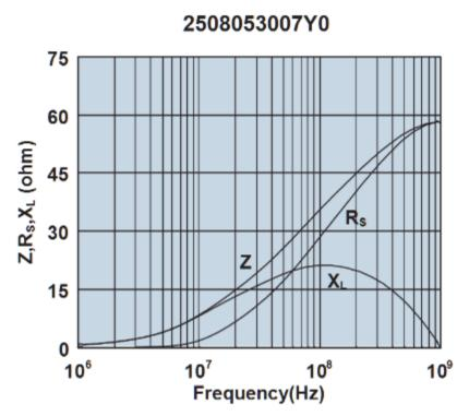
Impedance, reactance, and resistance vs. frequency.
