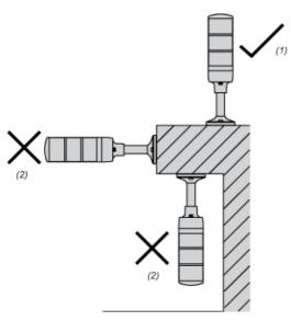
Choose a flat surface with enough strength and with little vibration for installation. Mount this product according to the figure to maintain IP characteristics.
