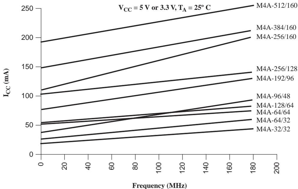
Figure 20. ispMACH 4A I<sub>CC</sub> Curves at Low Power Mode
