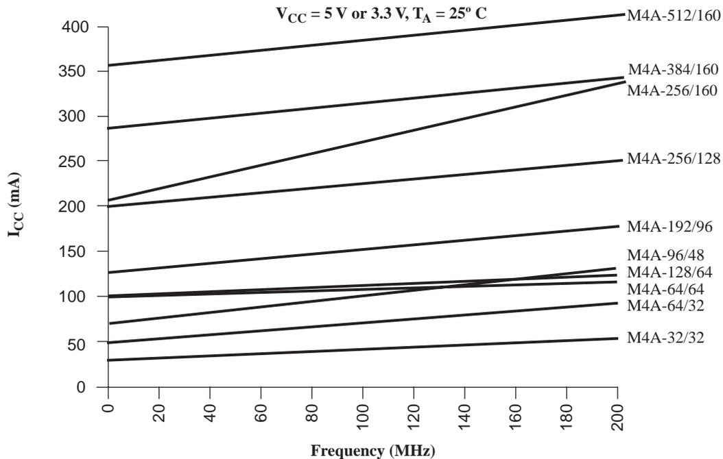
Figure 19. ispMACH 4A I<sub>CC</sub> Curves at High Speed Mode
