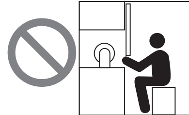
A person is between the sensor's detection zone and the hazardous zone of a machine.
