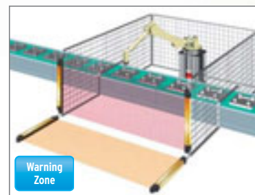
Dividing the zone between series-connected sensors
