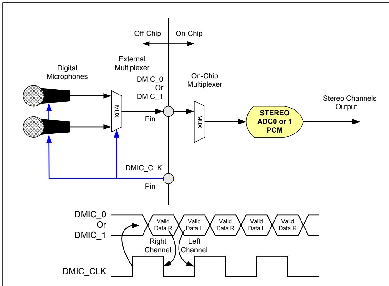
*Note: Some Digital Microphone Implementations support data on either edge, therefore, the external mux may not be required.*
