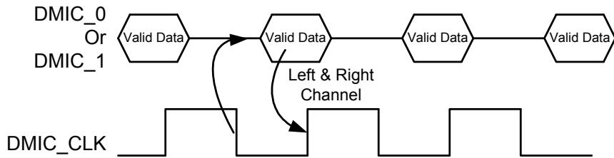
Figure 4. Stereo Digital Microphone Configuration
