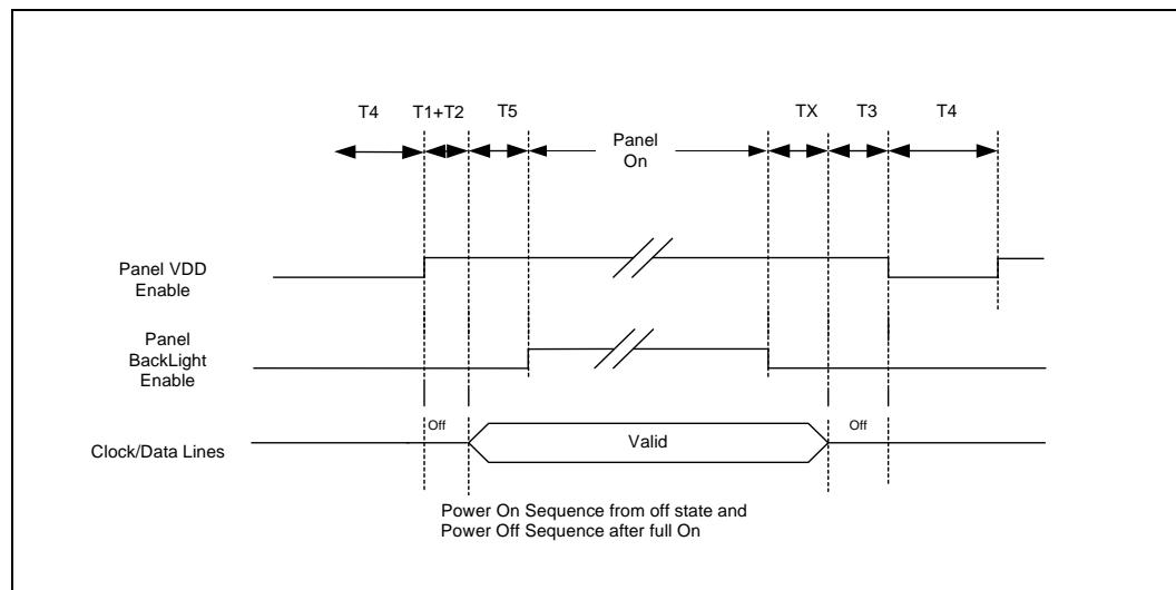
**NOTE:** Support for programming parameters TX and T1 through T5 using software is provided.
