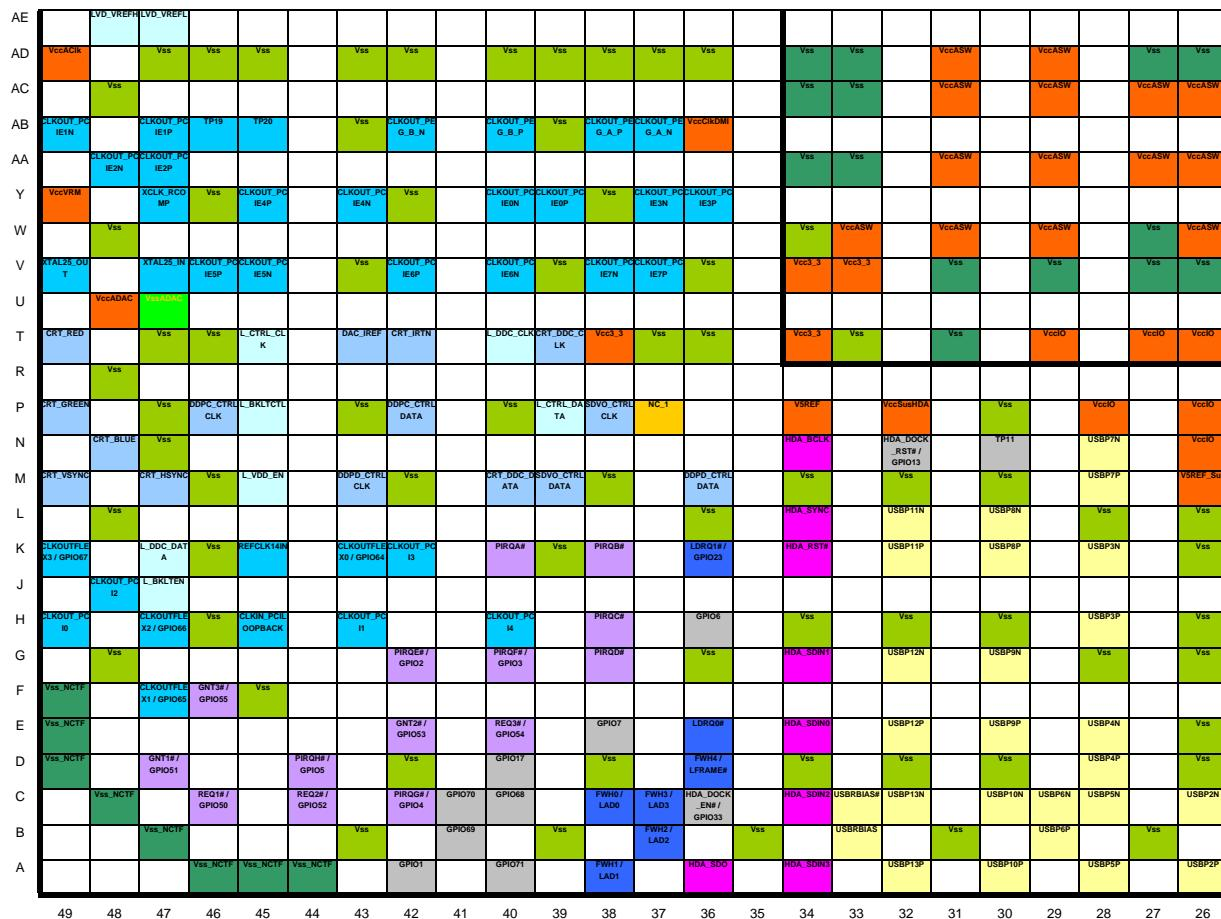
**Figure 6-7. Mobile PCH Ballout (Top View - Upper Right)**
