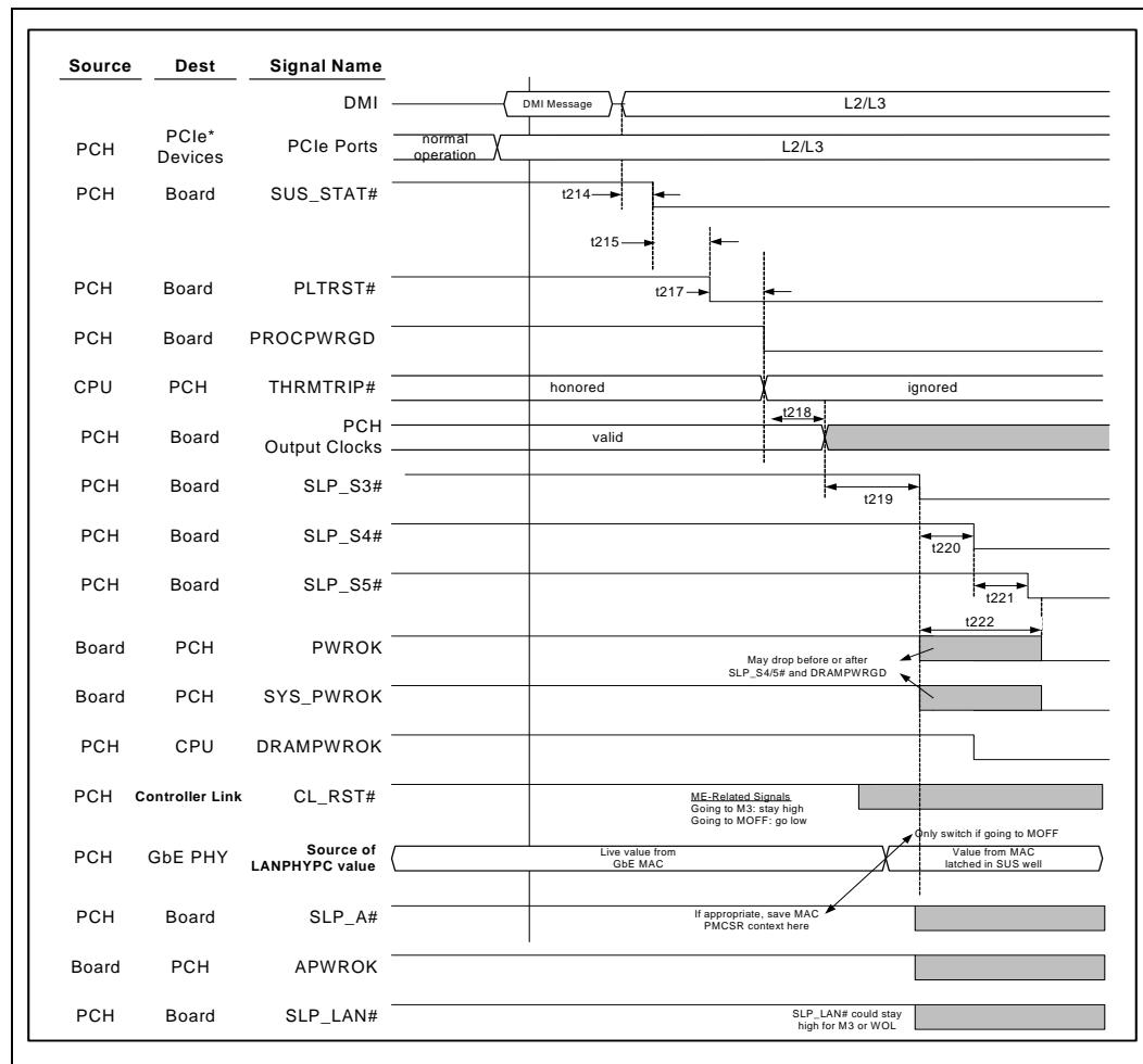
**Figure 8-7. S4/S5 to Deep S4/S5 to G3 w/ RTC Loss Timing Diagram**
