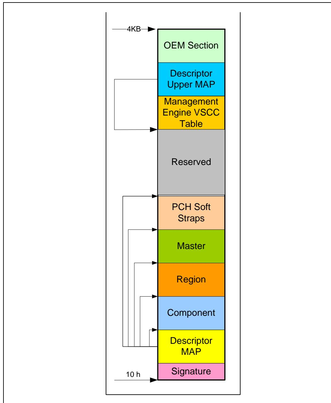
1. The Flash signature selects Descriptor Mode as well as verifies if the flash is programmed and functioning. The data at the bottom of the flash (offset 10h) must be 0FF0A55Ah in order to be in Descriptor mode.
