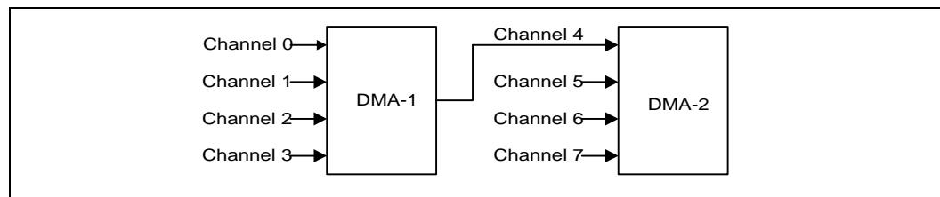
Each DMA channel is hardwired to the compatible settings for DMA device size:
