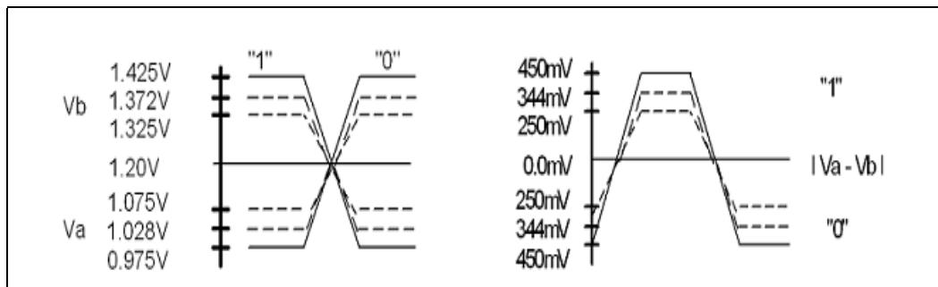
Logic values of 1s and 0s are represented by the differential voltage between the pair of signals. As shown in the [Figure 5-15](#) a serial pattern of 11000011 represents one cycle of the clock.
