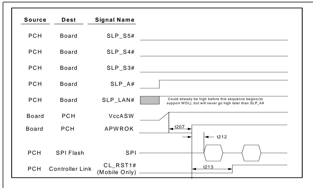
Figure 8-6. S0 to S5 Timing Diagram
