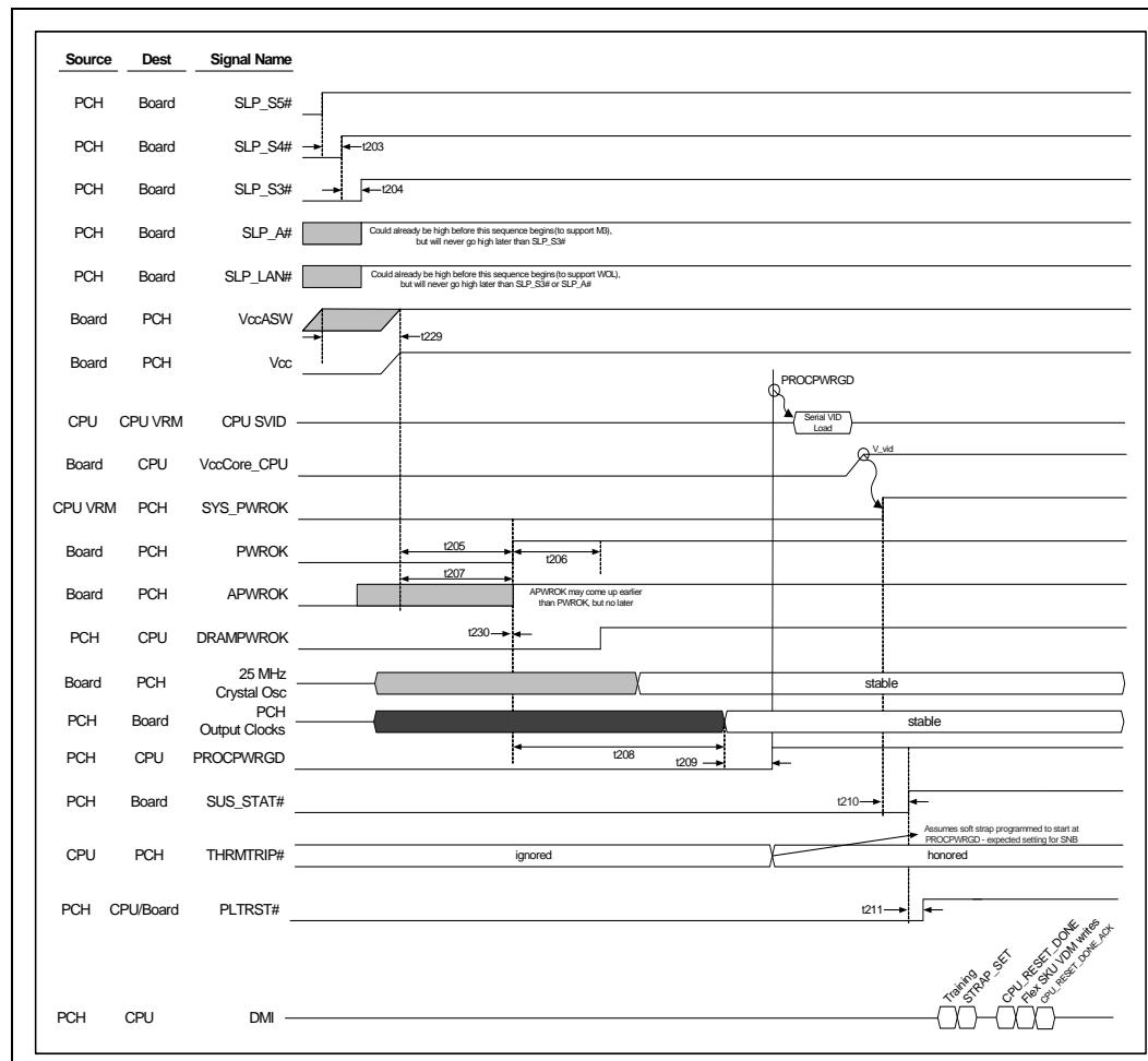
**Figure 8-4. S3/M3 to S0 Timing Diagram**
