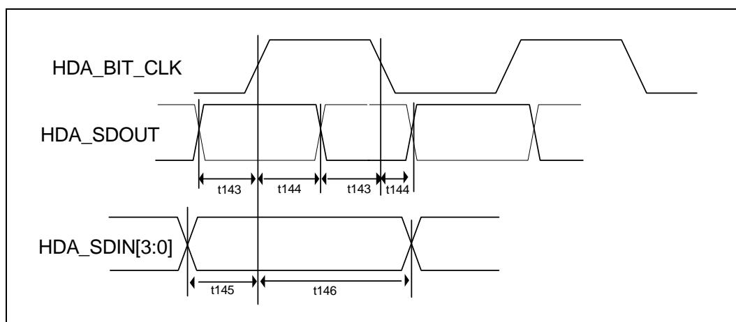
**Figure 8-24. Dual Channel Interface Timings**
