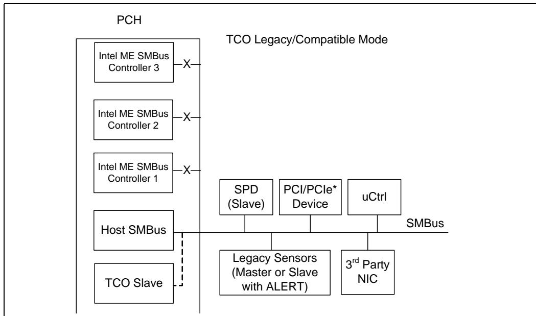
In TCO Legacy/Compatible mode the PCH can function directly with an external LAN controller or equivalent external LAN controller to report messages to a network management console without the aid of the system processor. This is crucial in cases where the processor is malfunctioning or cannot function due to being in a low-power state. [Table 5-39](#) includes a list of events that will report messages to the network management console.
