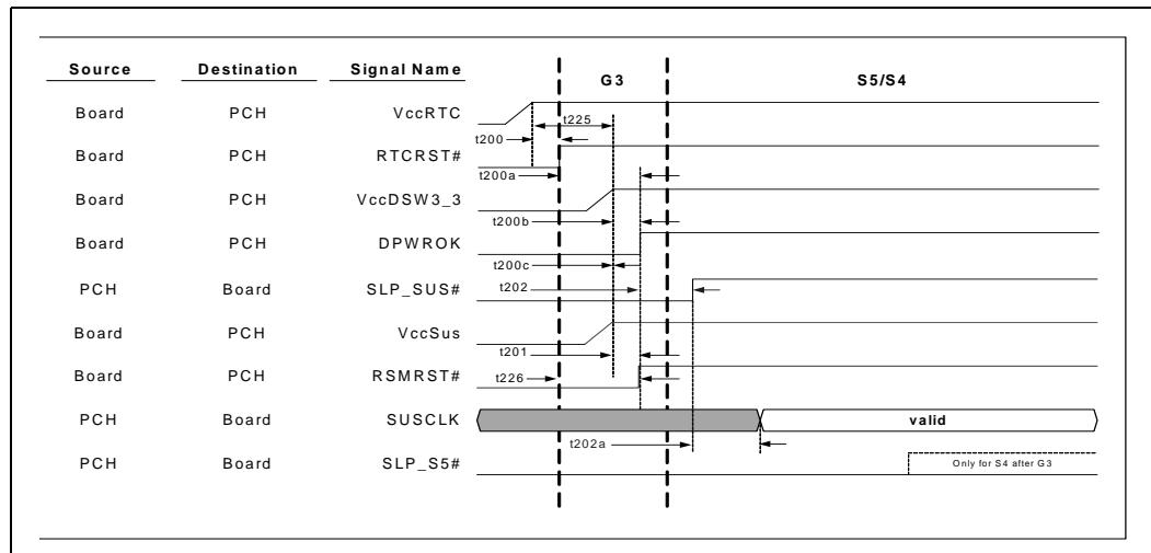
Figure 8-3. S5 to S0 Timing Diagram
