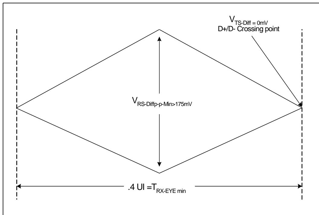
**Figure 8-30. Measurement Points for Differential Waveforms.**
