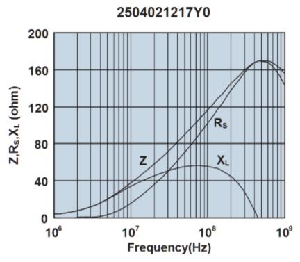
Impedance, reactance, and resistance vs. frequency.
