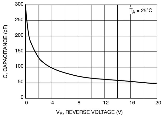
Figure 3. Typical Capacitance
