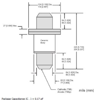
Package Capacitance  $(C_{\mu c}) =$
