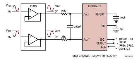
Figure 10. Fully-Differential Application Circuit
