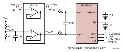
Figure 4. Pseudo-Differential Bipolar Application Circuit
