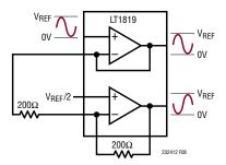
Figure 8. Single-Ended to Differential Driver
