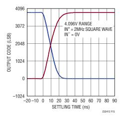
Figure 15. Transient Response of the LTC2324-12
