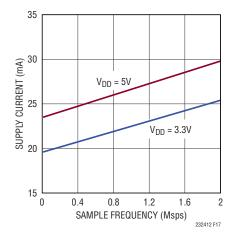
Figure 17. Power Supply Current of the LTC2324-12 vs Sampling Rate
