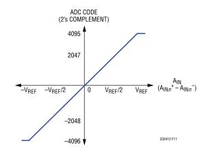
Figure 11. Fully-Differential Transfer Function
