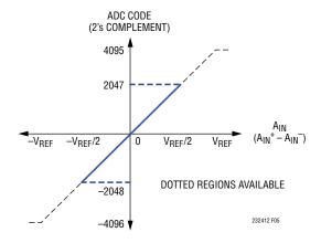
Figure 5. Pseudo-Differential Bipolar Transfer Function
