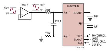
Figure 6. Pseudo-Differential Unipolar Application Circuit
