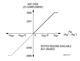
Figure 7. Pseudo-Differential Unipolar Transfer Function
