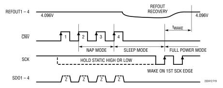
Figure 18. CMOS Mode SLEEP and WAKE Using SCK
