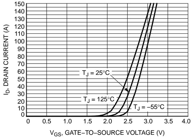
Figure 2. Transfer Characteristics
