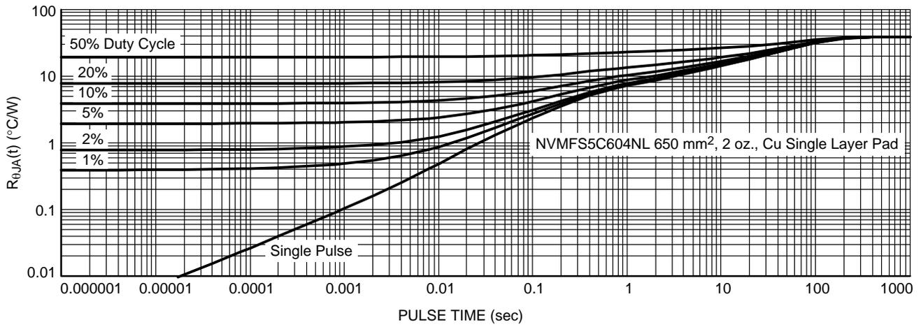
Figure 13. Thermal Characteristics
