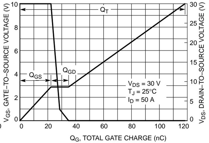
Figure 8. Gate-to-Source and Drain-to-Source Voltage vs. Total Charge
