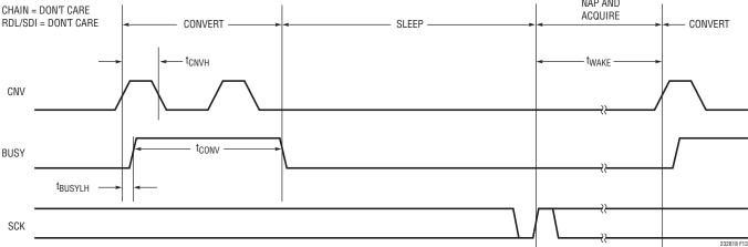
Figure 13. Sleep Mode Timing Diagram
