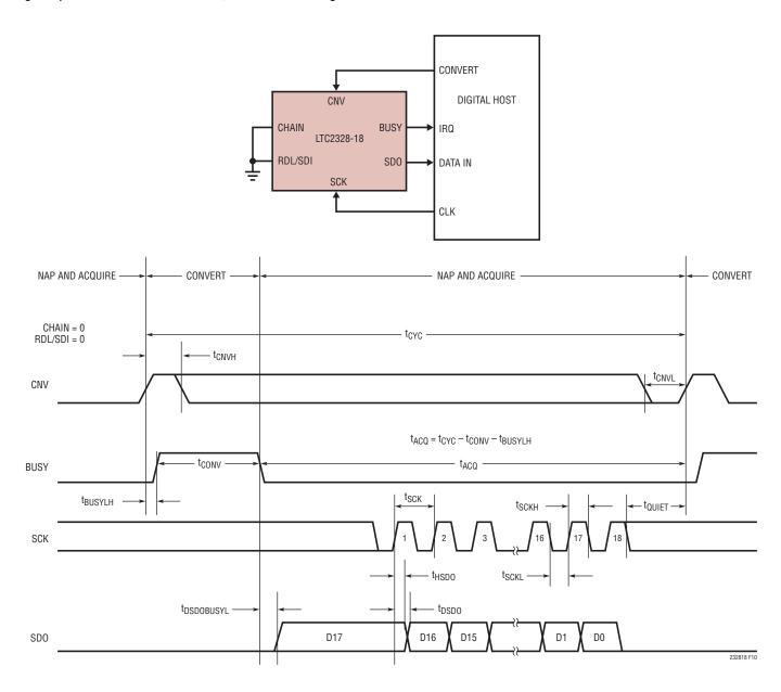
Figure 10. Using a Single LTC2328-18 in Normal Mode
