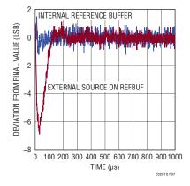
Figure 7. Transient Response of the LTC2328-18
