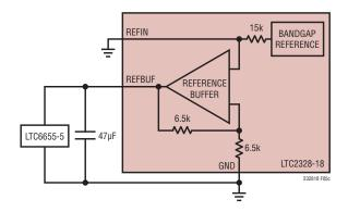
Figure 5c. Overdriving REFBUF Using the LTC6655-5
