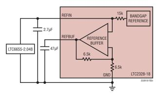
Figure 5b. Using the LTC6655-2.048 as an External Reference
