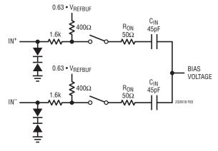
Figure 3. The Equivalent Circuit for the Differential Analog Input of the LTC2328-18
