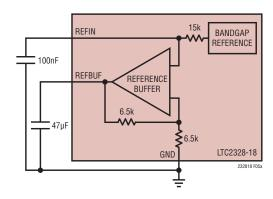
Figure 5a. LTC2328-18 Internal Reference Circuit
