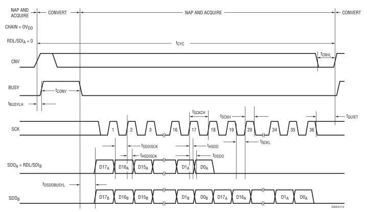
Figure 12. Chain Mode Timing Diagram
