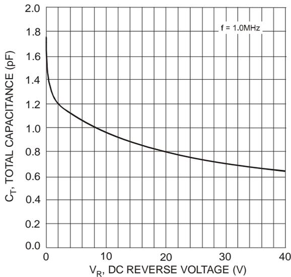
Fig. 3 Total Capacitance vs. Reverse Voltage, Per Element
