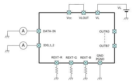
Test Circuit 3 Supply Current (VL)
