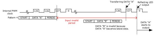
The period between DATA "A" period end and the second rising edge of zero internal PWM clocks is the input invalid period. Therefore, DATA "B" is invalid and DATA "A" is output.
