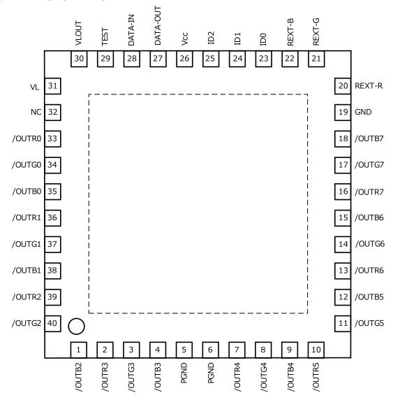
Please be sure to connect the back radiation PAD of a QFN package to GND of a substrate.
