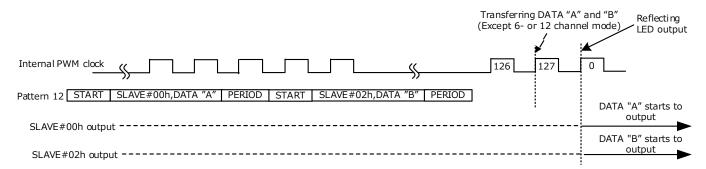
Both DATA "A" and DATA "B" are output at the rising edge of zero internal PWM clock which is just after DATA "A" and DATA "B" inputs.
