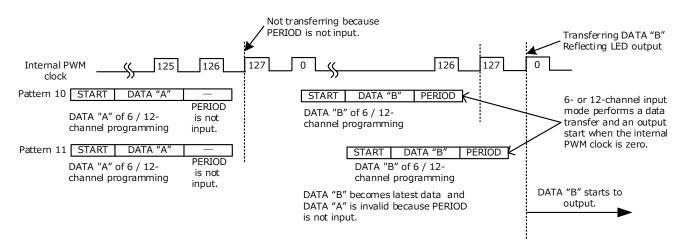
DATA "B" starts to output at the rising edge of zero internal PWM clocks if the period of DATA "A" is not input and the period of next DATA "B" is input.
