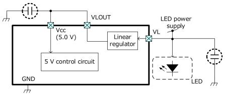
As shown in the above, the power supply (7.0 to 28 V) is applied to the VL pin, and VOUT and Vcc pins are connected directly.
