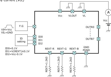
Test Circuit5 Output Current / Output Leakage Current / Output Current Accuracy / Changes in Constant Output current dependent on Vcc
