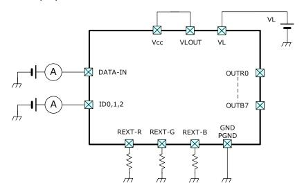
Test Circuit 2 Input Current (IIL)
