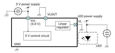
When 5 V power supply is applied to this product without using the built-in power supply, ground VL pin and VLOUT pin to GND.
