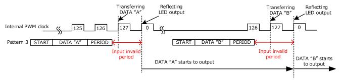
DATA "A" starts an output at the rising edge of zero internal PWM clocks just after DATA "A" period. Then DATA "B" starts an output at rising edge of zero internal PWM clocks just after DATA "B" period.
