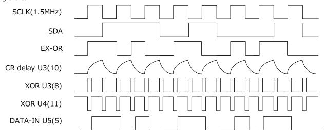
Note: When this circuit is used, the interval period should be fixed to SDA=SCLK=High.
