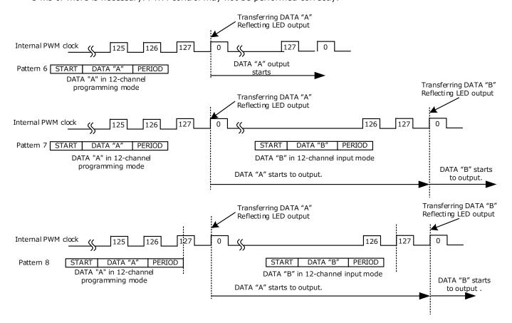
Since there is no input invalid period, an input data are started to output at the rising edge of the first zero internal PWM clocks after inputting the period command.
