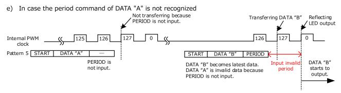
When the period of DATA "A" is not input and the period of next DATA "B" is input, DATA "B" starts output immediately after at the rising edge of zero internal PWM clocks.
