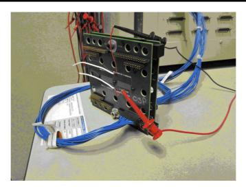
Figure 3 LLCR Measurement Points
