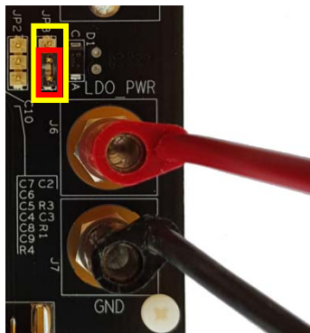
Figure 10. External Power Configuration
