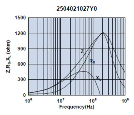
Impedance, reactance, and resistance vs. frequency.
