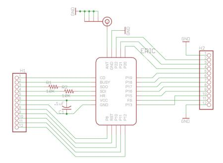
Note the 10k series resistors fitted to the SDO & SDI pins. Other eRIC pins (configured as inputs) may need to be similarly protected if connected to external 5V logic level signals.
