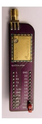
This board assembly 'breaks out' the 5 x 7 pins of the eRIC RF Transceiver to a more convenient  $2 \times 12 \times 0.1$ " pitch DIL pinout that matches commercial prototype breadboards. This allows the quick and easy testing and evaluation of eRIC modules for which these boards are intended.
