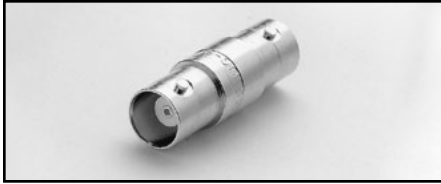
CS-565: Female BNC to female BNC adapter with 50Ω nominal impedance. For use with: 4200-SCS, BNC interconnect
