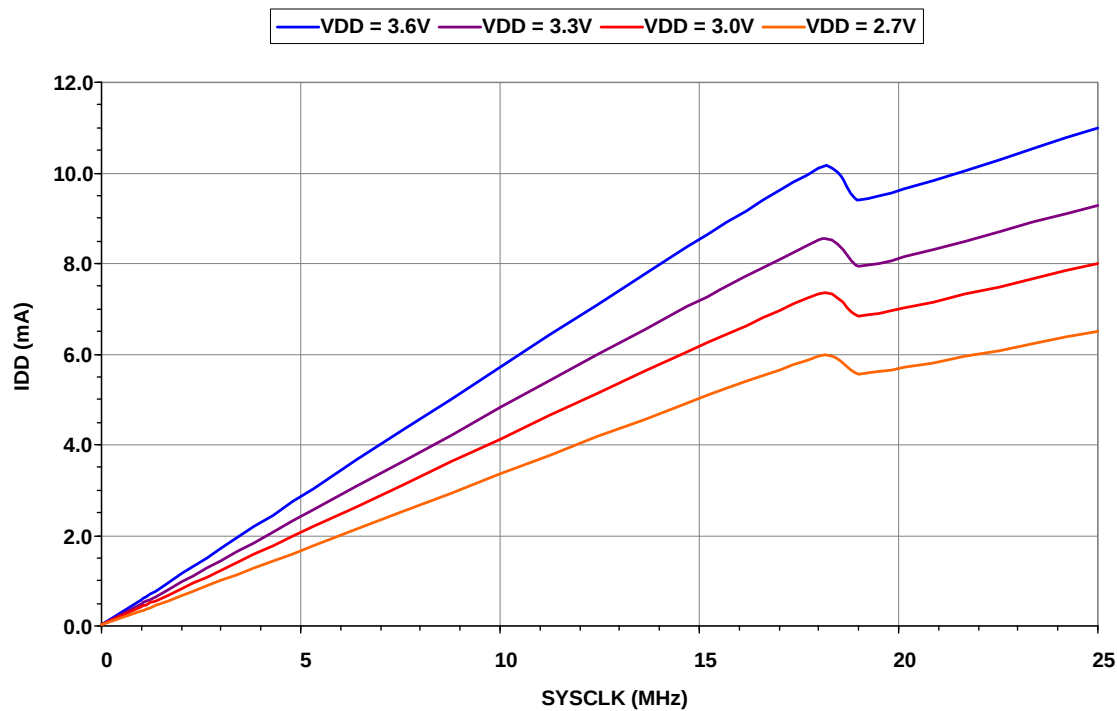
Figure 6.1. Normal Mode Digital Supply Current vs. Frequency
